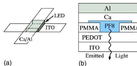
FIG. 2. (Color online) Schematic drawing of a working PF8 LED design as fabricated with the microplotter: (a) general spatial layout and (b) vertical layout.
