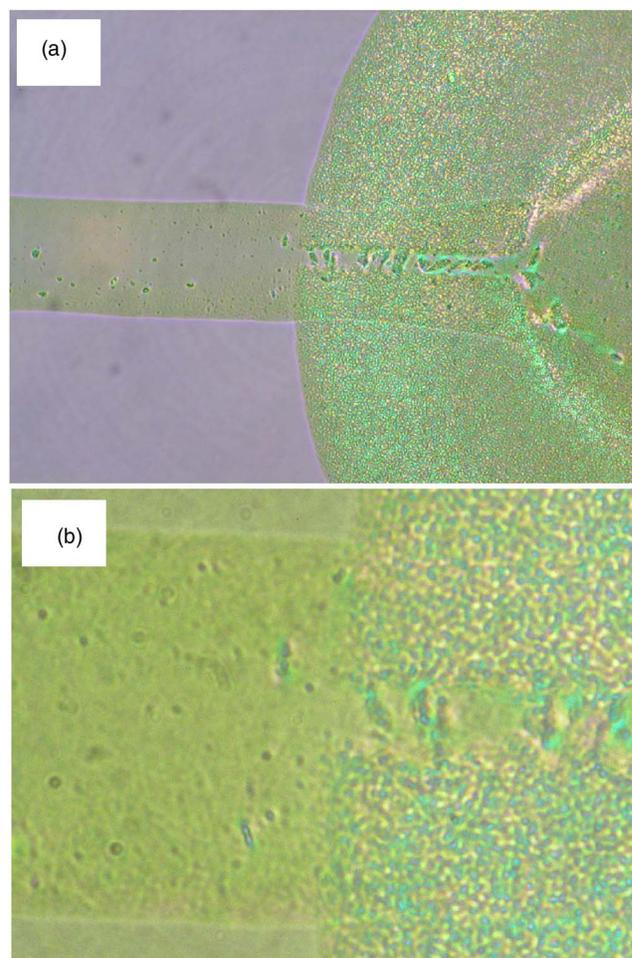
FIG. 4. (Color online) Polarizing optical microscope images (at two magnifications) of a microplotter trace at the position of initial deposition.
