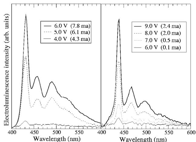
FIG. 9. Example electroluminescence spectra from two different PLED devices operated at the indicated voltages.
