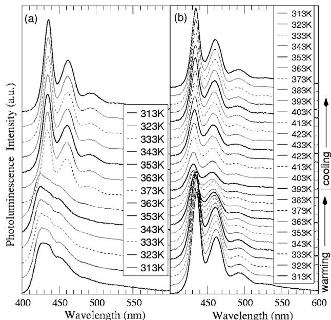
FIG. 7. Temperature dependent PL spectra from film deposited at  $1000 \mu\text{m/s}$  (from 2% w/w PF8/CB solution) on thermal cycling: (a) from 313 K (bottom) up to 373 K (middle) and back down to 313 K (top); (b) same film on second thermal cycle from 313 K (bottom) up to 433 K (middle) and back down to 313 K. All spectra have been offset and rescaled for clarity.
