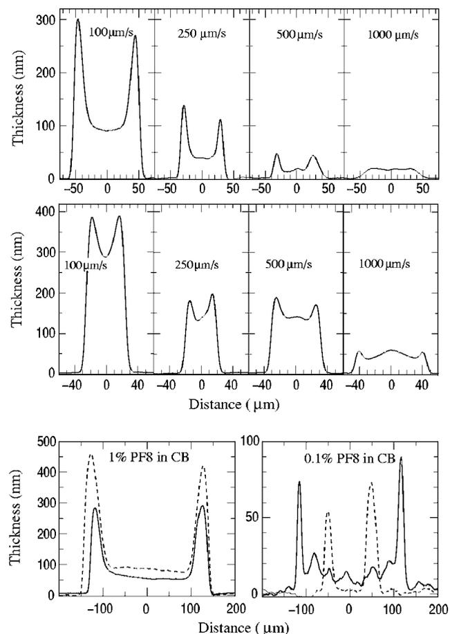
FIG. 5. Profilometer traces of PF8 thin film lines as fabricated by the microplotter at as indicated tip speeds. The widths range from 50 to 100  $\mu\text{m}$  and the large rise in film thickness at the fluid contact line is most pronounced at low deposition speeds. Top: lines formed using 1% w/w PF8/CB solution. Middle: lines formed using 2% w/w PF8/CB solution. Bottom: Profilometer traces of PF8 thin films produced by drop casting from the indicated PF8/CB solutions.
