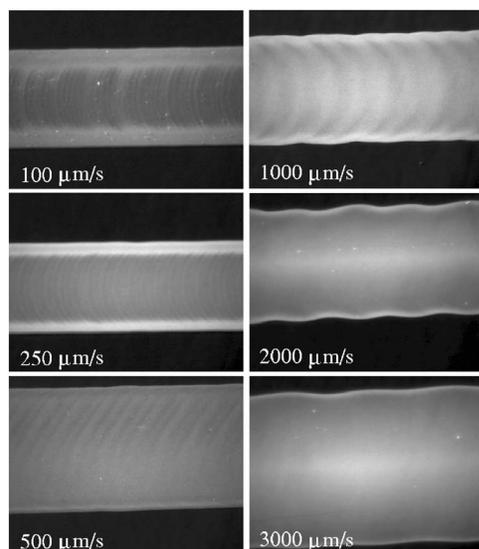
FIG. 3. Fluorescence microscopic images of individual microplotter traces at as indicated tip speeds.
