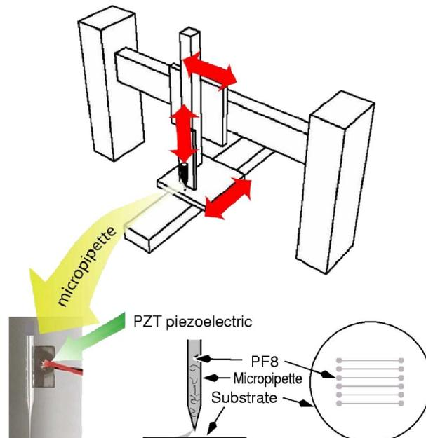
FIG. 1. (Color online) Top: schematic layout of the XYZ microplotter system that provides micron positional precision. Bottom: a photograph of the micropipette/piezoelectric crystal assembly and a typical test pattern of 1 cm long lines on the sapphire substrate.
